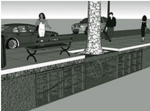
Diagram of a covered soil area with structural cells (Source: caseytrees.org)
