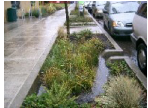
Examples of tree wells that function as water quality/management facilities (bio-swales), pedestrian safety features, & visual amenities
