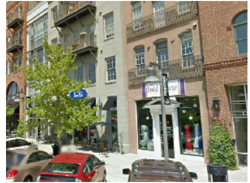
An example of well-shielded street lighting, placed in proper relation to street trees and other streetscape standards
