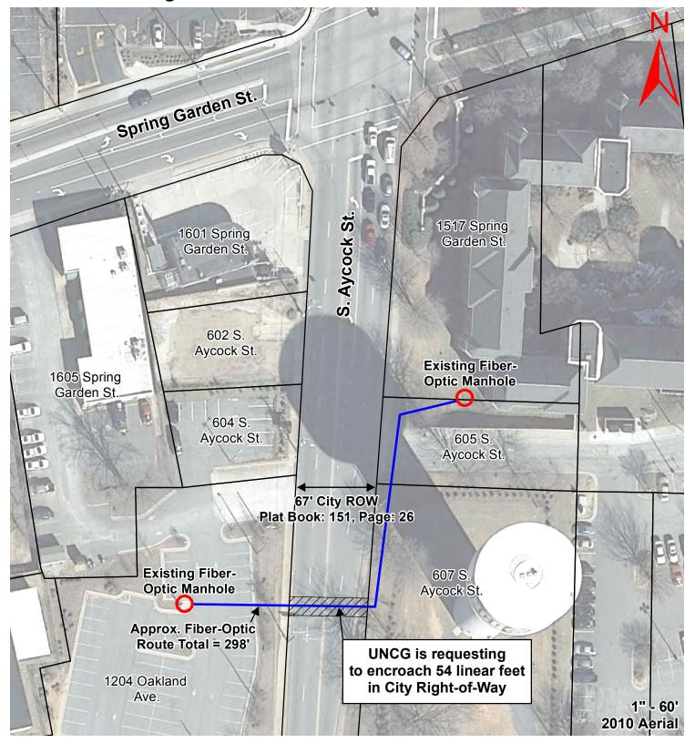
SITE PLAN WITH PROPOSED ENCROACHMENT IN CITY RIGHT-OF-WAY For UNCG
